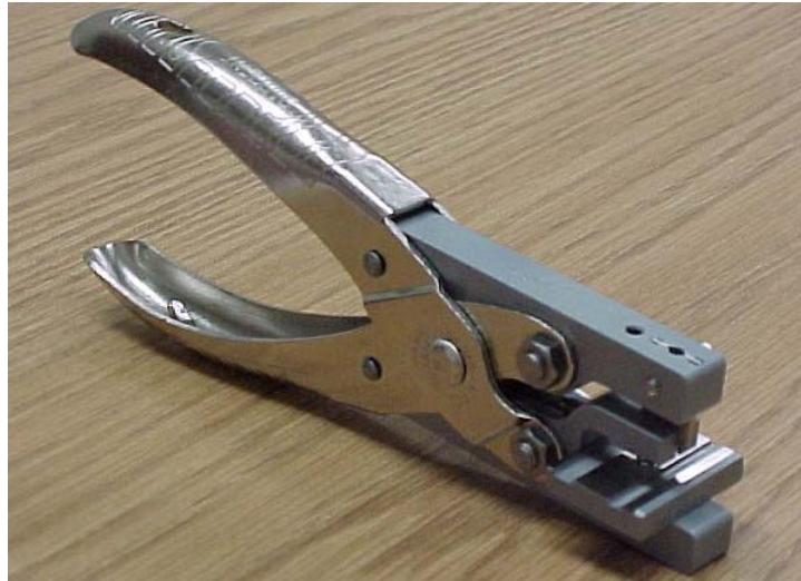
Figure 24 BPY75D37 Wire Insertion Repair Tool
