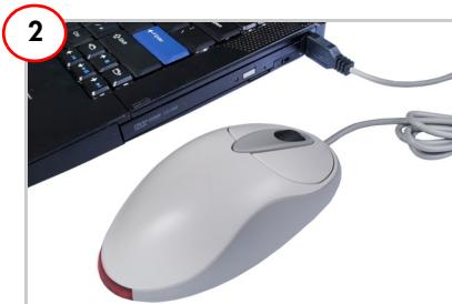
Connect the mouse to the PC through the USB. The mouse enumerates as a HID device.
