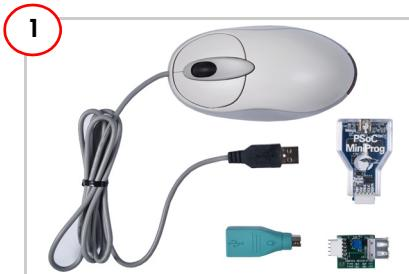
Unpack the mouse, MiniProg, USB-to-PS2 converter, and the USB-to-ISSP programming adapter.
