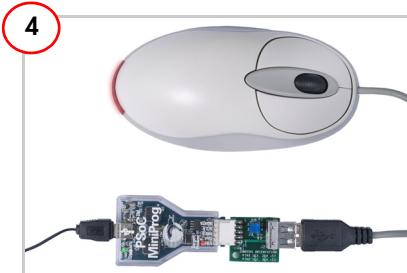
To program the mouse, connect the USB-to-ISSP programming adapter to the USB connector of the mouse.
