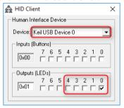
To test the functionality of the USB HID device run the *HIDClient.exe* utility and follow these steps:
