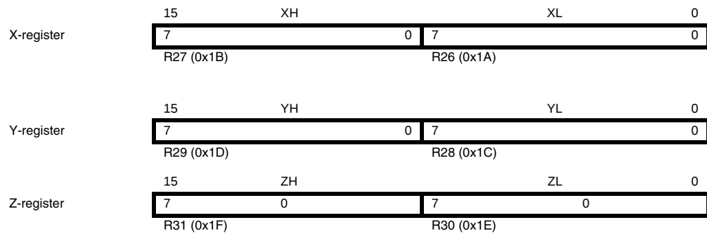
Figure 7-3. The X-, Y-, and Z-registers
