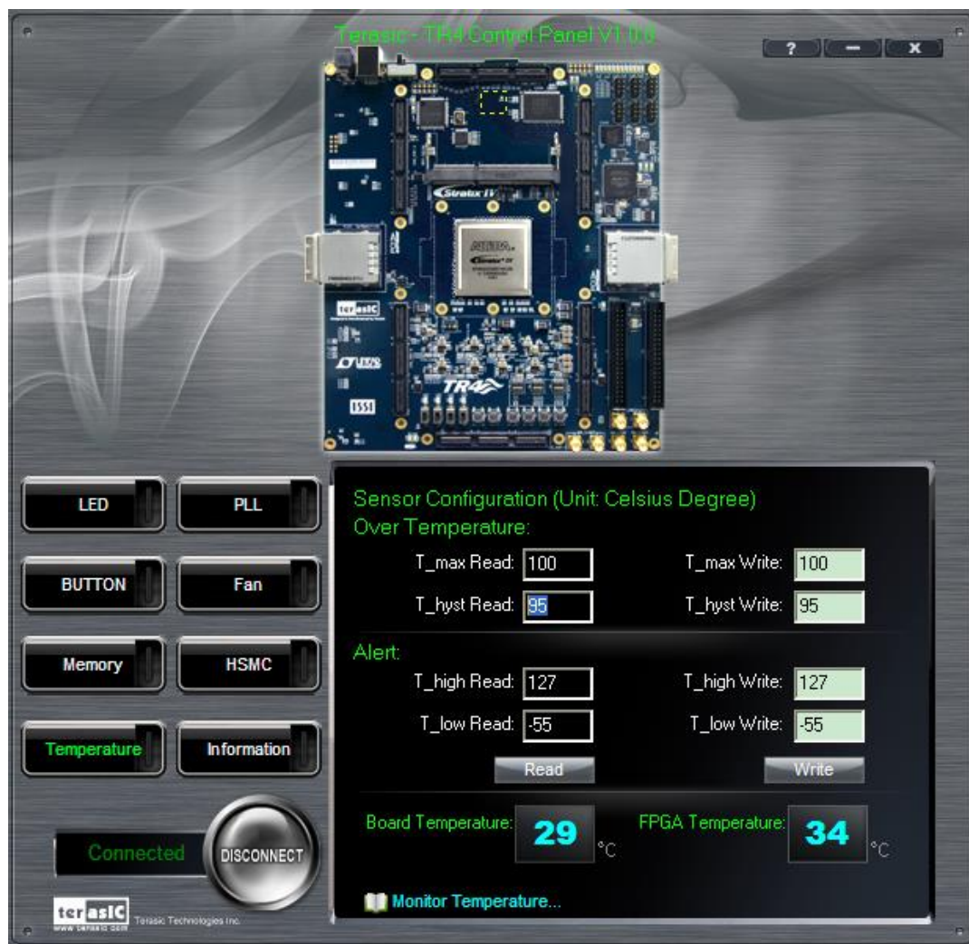
Figure 3-9 Accessing the Temperature Sensor through Control Panel
