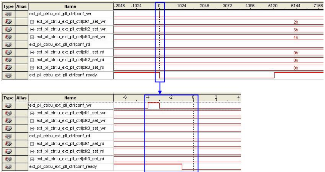
Figure 5-3 Write Timing Waveform
