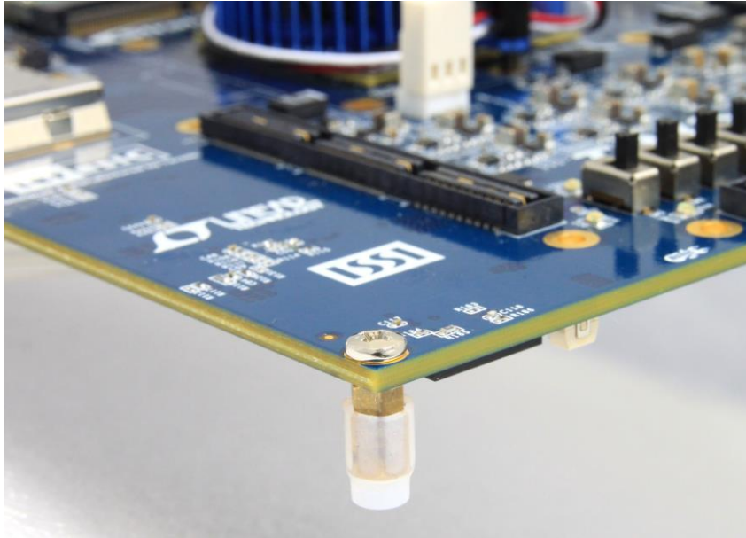
Figure 1-4 Mount Silicon Foot Stands
