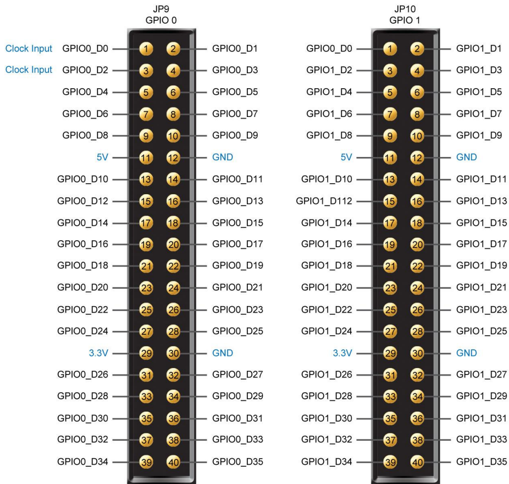
Figure 2-21 Pin Distribution of the GPIO Expansion Headers
