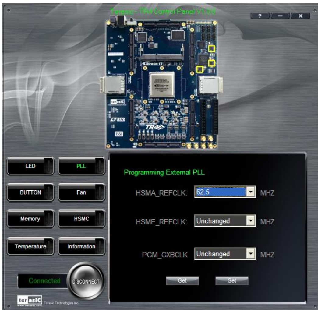
Figure 3-10 Programmable External PLL Configured through Control Panel
