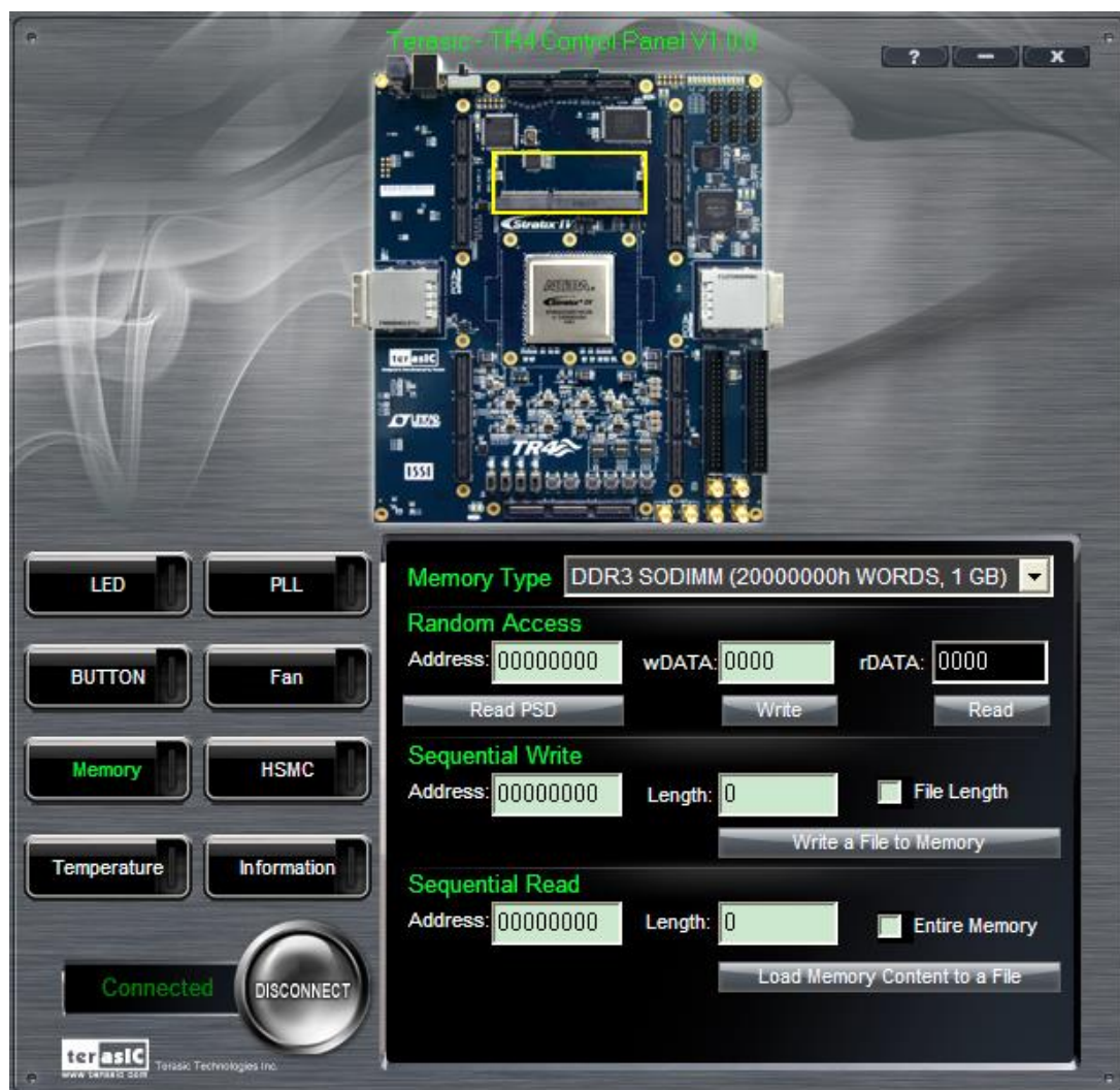
Figure 3-7 Access DDR3 SO-DIMM Memory
