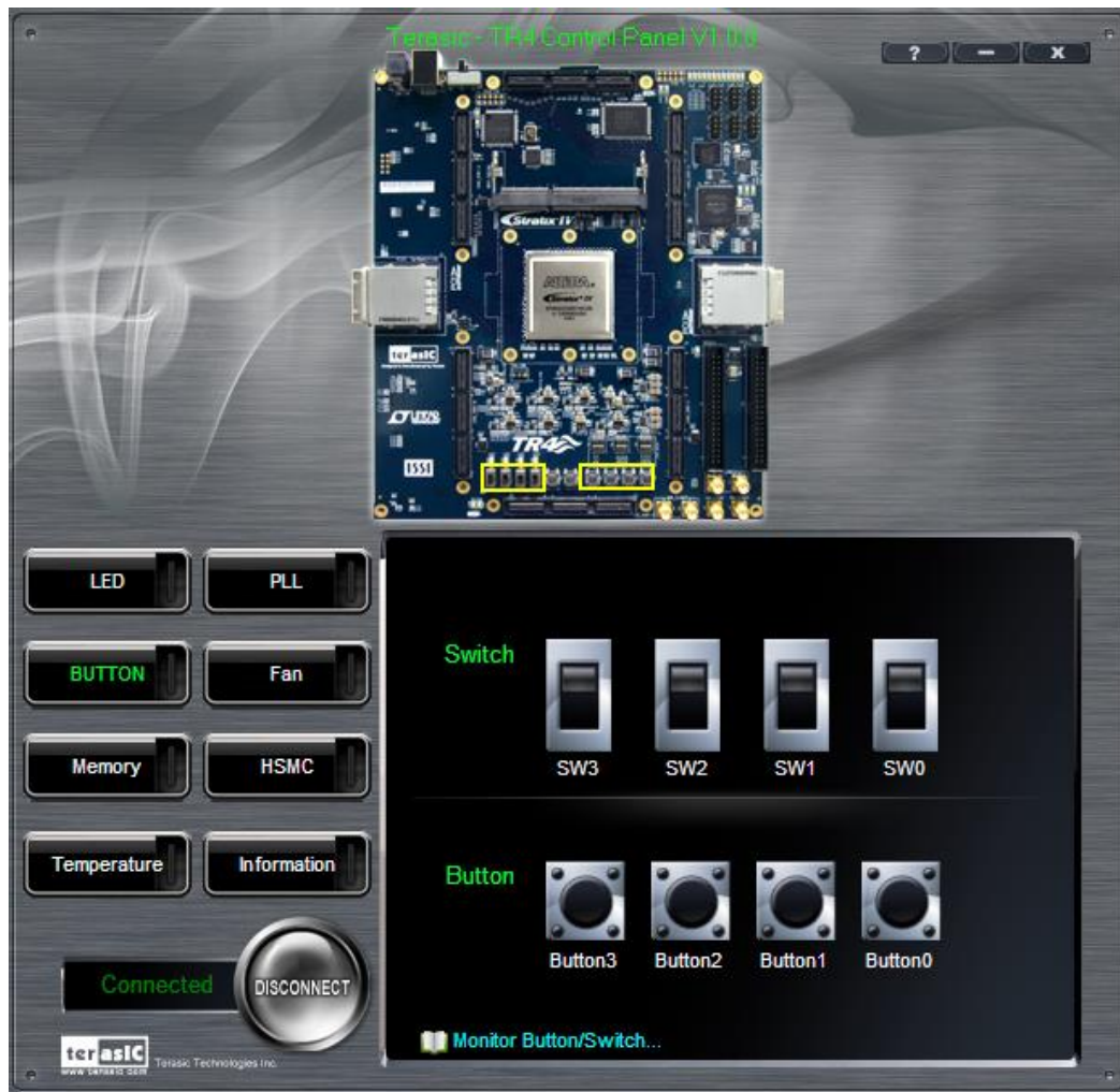
Figure 3-6 Monitoring Switches and Buttons
