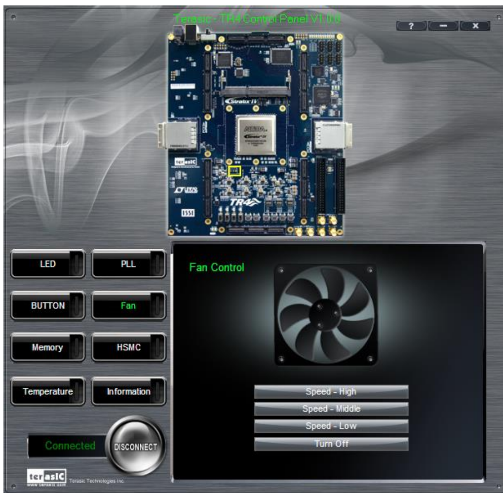
Figure 3-12 Fan Control of the TR4
