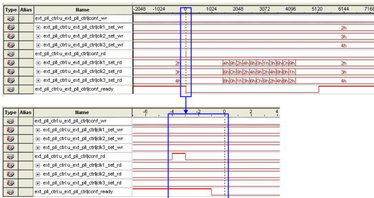
Figure 5-4 Read Timing Waveform
