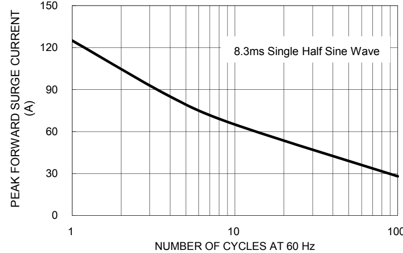
FIG. 3 MAXIMUM NON-REPETITIVE FORWARD SURGE CURRENT
