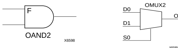
Figure 20: AND & MUX Symbols in XC4000X IOB
