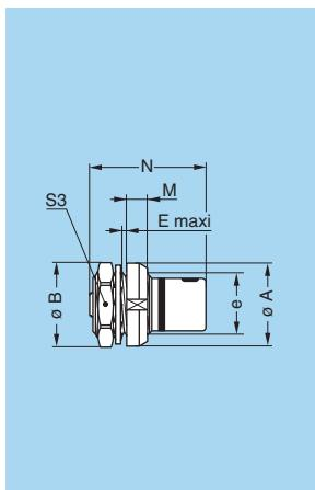
**EC● Fixed socket with 2 nuts, key (N) or key (S), protruding shell, IP50 (back panel mounting)**
