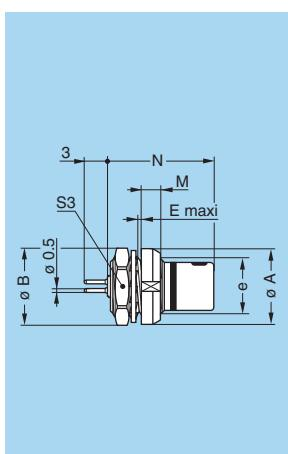
**EC● Fixed socket with 2 nuts, key (N) or key (S), protruding shell, print contacts, IP50 (back panel mounting)**
