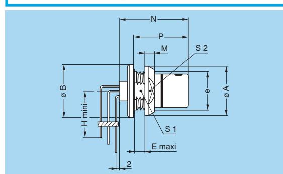
**HE● Fixed socket, nut fixing, key (N) or key (P), with elbow (90°) contacts for printed circuit, (back panel mounting)**
