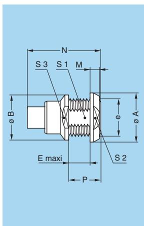
**EE● Fixed socket, nut fixing, key (N) or keys (P, S and T), IP50 (back panel mounting)**
