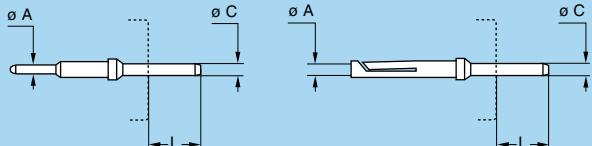
Print elbow contacts include a tinned copper wire crimped into a contact.
