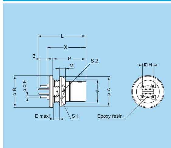
**HE● Fixed socket, nut fixing, key (N) or keys (P, S, T, W and X), for printed circuit, (back panel mounting)**
