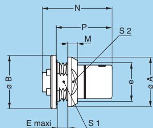
**EH● Fixed socket, nut fixing, key (N) or keys (P, S, T, W and X), (back panel mounting)**
