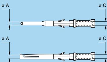
A detailed range of conductor dimensions that can be crimped into our contacts is given on the table at right. See also the section on tooling (pages 30 to 33).
