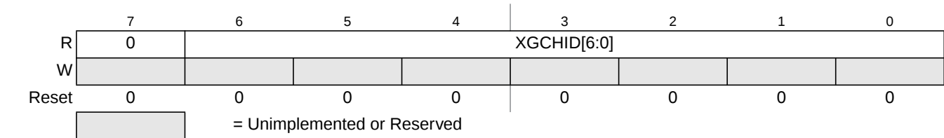
Figure 6-4. XGATE Channel ID Register (XGCHID)
