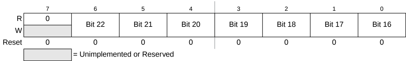
Figure 20-15. Debug Comparator Address High Register (DBGXAH)
