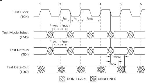
TAP AC Switching Characteristics Over the operating Range<sup>[3, 4]</sup>
