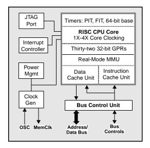
The CPU core handles instruction decoding and execution. The instruction cache unit passes instructions to the queue in the CPU core or, in the event of a cache miss, requests a fetch from external memory through the bus control unit.
