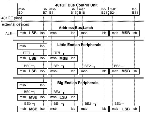
The 401GF external bus pins used for address output and data transfers are shown in the table below. Address bits output by the 401GF are numbered A0:31, with A0 as the most significant bit (msb).
