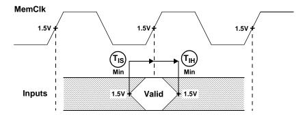
**Table 13. 401GF Synchronous Input Timings**
