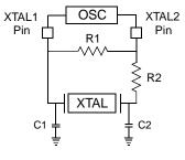
R2 functions as a current limiting resistor to the crystal, and also as an oscillation stabilizer in the presence of perturbations induced by moisture, component variations, or other factors.
