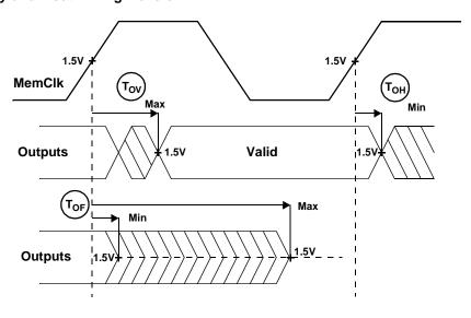
Table 15. 401GF Synchronous Output Timings
