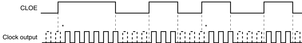
Figure 12-4. Remote Control Output Application Example
