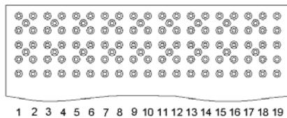
Recommended PCB hole mounting pattern for row differential
