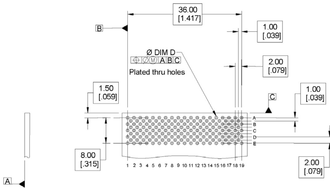
Recommended PCB hole mounting pattern for coaxial,
