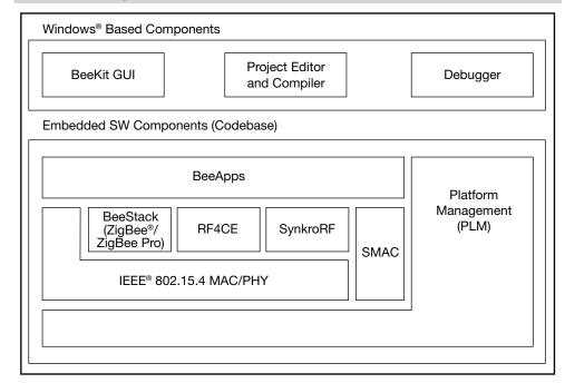
ZigBee technology provides the ideal solution for larger, more complex networking, a robust and reliable option for self-forming and self-healing mesh networks. Since ZigBee is an open standard, it also allows for interoperability of products from different vendors. BeeStack is Freescale's ZigBee protocol stack that delivers a reliable and robust platform for ZigBee development.
