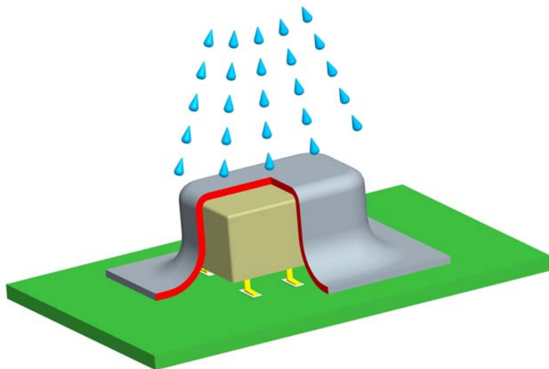
Fig. 11: Coating of relays on PCB's
