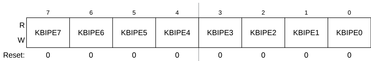
Figure 7-4. KBIX Pin Enable Register
