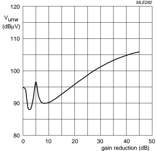
$V_{DS}$  = 5 V;  $V_{GG}$  = 5 V;  $R_{G1}$  = 150 kΩ;  $f$  = 50 MHz;  $f_{unw}$  = 60 MHz;
