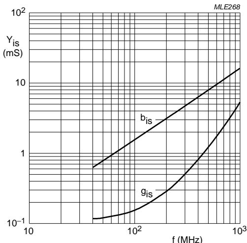
$V_{DS} = 5$  V;  $V_{G2} = 4$  V;  $I_D = 18$  mA;  $T_{amb} = 25$  °C.
