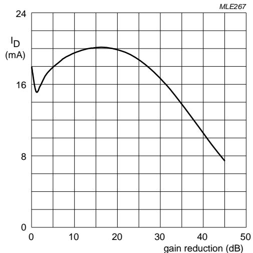
$V_{DS}$  = 5 V;  $V_{GG}$  = 5 V;  $R_{G1}$  = 91 kΩ;  $f$  = 50 MHz;  $T_{amb}$  = 25 °C;
