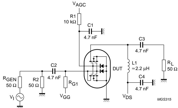
Fig.35 Cross-modulation test set-up (for one MOS-FET).
