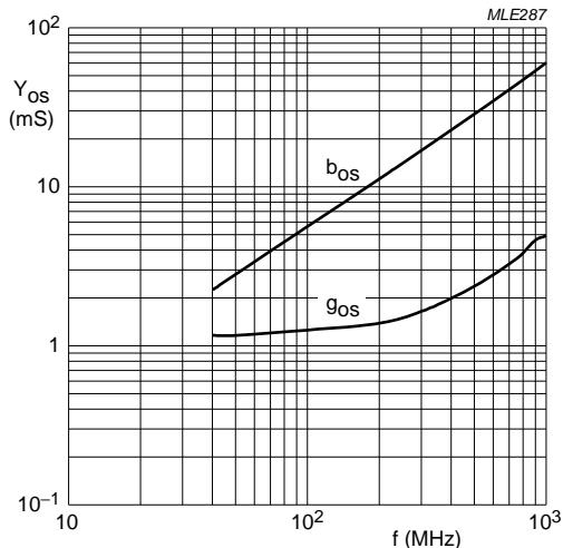
$V_{DS} = 5$  V;  $V_{G2} = 4$  V;  $I_D = 12$  mA;  $T_{amb} = 25$  °C.
