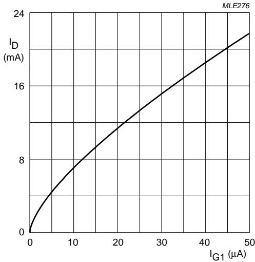
$V_{DS} = 5 \text{ V}$ ;  $V_{G2-S} = 4 \text{ V}$ ;  $T_j = 25 \text{ }^\circ\text{C}$ .
