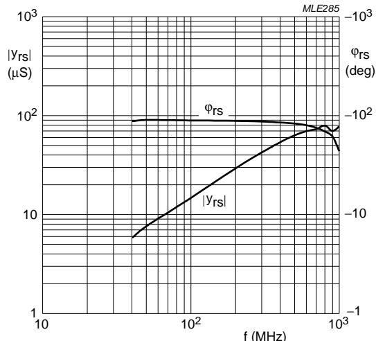
$V_{DS} = 5$  V;  $V_{G2} = 4$  V;  $I_D = 12$  mA;  $T_{amb} = 25$  °C.
