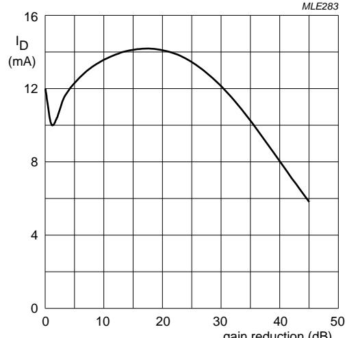
$V_{DS}$  = 5 V;  $V_{GG}$  = 5 V;  $R_{G1}$  = 150 kΩ;  $f$  = 50 MHz;  $T_{amb}$  = 25 °C;
