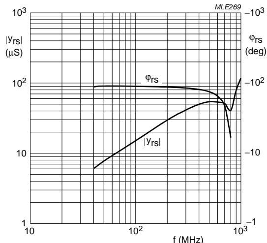
$V_{DS} = 5$  V;  $V_{G2} = 4$  V;  $I_D = 18$  mA;  $T_{amb} = 25$  °C.
