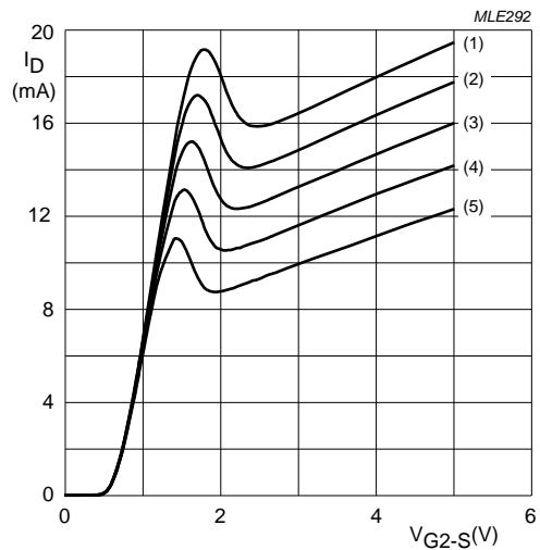
$V_{DS} = 5$  V;  $T_j = 25$  °C;  $R_{G1} = 91$  kΩ (connected to  $V_{GG}$ ); see Fig.35.
