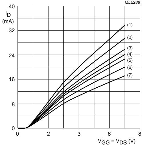
$V_{G2-S} = 4$  V;  $T_j = 25$  °C;  $R_{G1} = 150$  kΩ (connected to  $V_{GG}$ ); see Fig.35.
