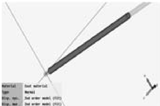
Figure 7. Microwave CST Model of Cable with Q-Zorb Coating
