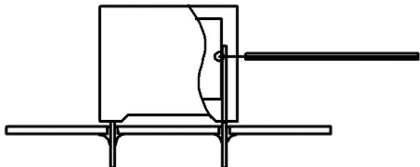
Temperature monitored inside the capacitor.
