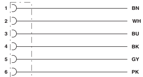
Contact assignment of M8 socket
