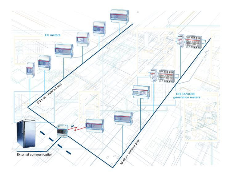
The EQ meter gateway is used as an access point to all of the EQ meters and allows the user to perform settings using high level programming language JSON or through a web browser. When safety and maximum functionality is of importance the EQ bus will make it fully utilized over the EQ meter gateway. Meters with RS-485 can be used for Modbus or EQ bus.
