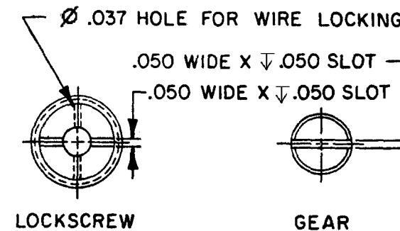
LEVER MAY BE ADJUSTED FOR AN INFINITE NUMBER OF POSITIONS THRU 360°. ADJUSTMENT IS MADE BY LOOSENING THE LOCK NUT AND THEN THE LOCKSCREW AND TURNING GEAR UNTIL LEVER IS IN DESIRED POSITION. LOCKSCREW AND LOCK NUT ON SHAFT IS THEN TIGHTENED TO POSITIVELY LOCK LEVER IN POSITION.
