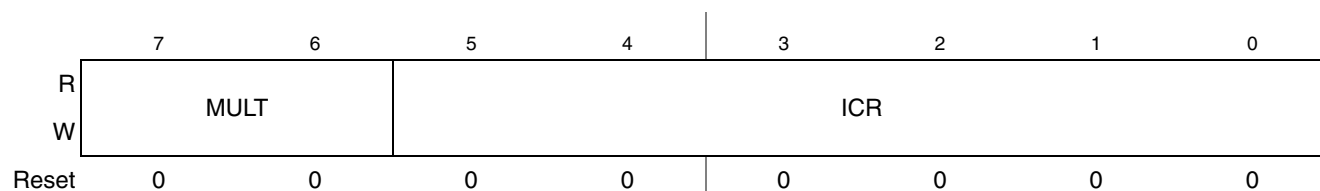
Figure 11-4. IIC Frequency Divider Register (IICF)
