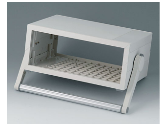
B2211317 MEDITEC D 160, with handle bar ABS (UL 94 HB) off-white RAL 9002 11.42"x7.87"x4.88" IP 40
