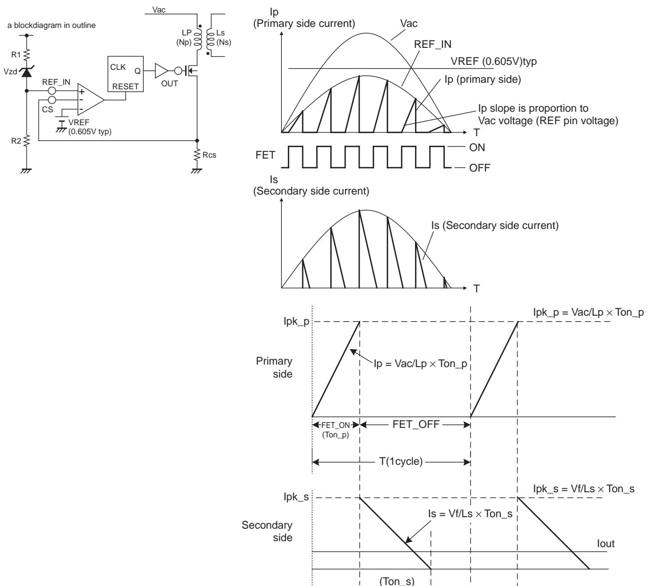
[Inductance  $L_p$  of primary side and sense resistor  $R_s$ ]
