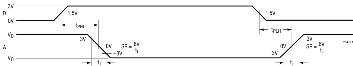
Figure 15. V.28 Driver Propagation Delays
