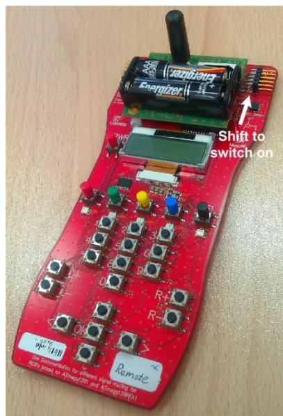
Figure 7-3. Assembled RCB Hosted on a Key Remote Control Board
