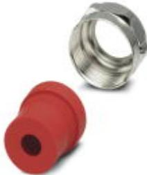
Half screw connection Pg21, made of metal, consisting of rubber seal with one hole and one pressure screw, for type 2 - 4 housings, cable [mm] 9 - 13
