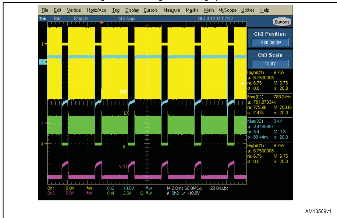
Figure 25: Inverting BB dimming operation
