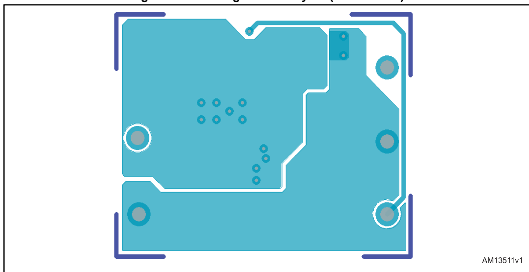
Figure 27: Inverting BB PCB layout (bottom side)
