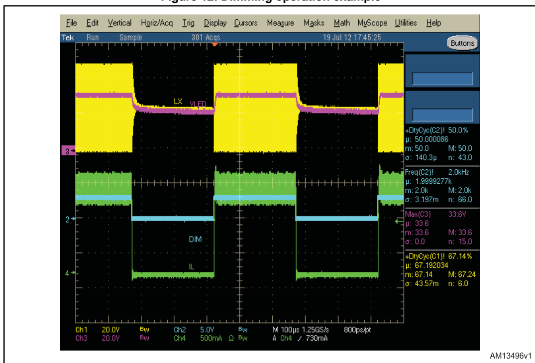
Figure 12: Dimming operation example
