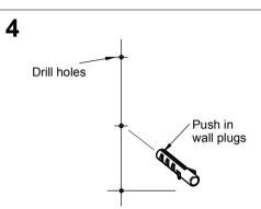
Where marked, drill a hole for each wall clip using a 6mm drill bit to a depth of 35mm. Insert a wall plug into each hole so that they are flush with the wall surface.
