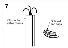
Finally push on the cable covers so that they clip into place. If cables enter or exit through a hole in the wall, you may push-in one or both of the plastic end caps.
