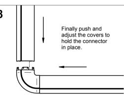
Hold the corner connector roughly in place and slide the cable covers towards it so that they push over the protruding lugs. Adjust the covers position until they sit flush.
