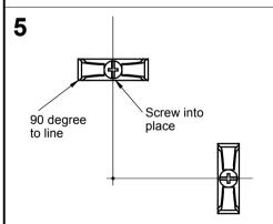
Screw each wall clip into place using a cross head screwdriver. Ensure they are central to the lines and sitting across them at 90 degrees as shown.
