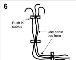
Push cables through the gap in the front of the wall clips so they are retained. Use the cable ties to help group the cables at points in between the wall clips. Trim off excess.
