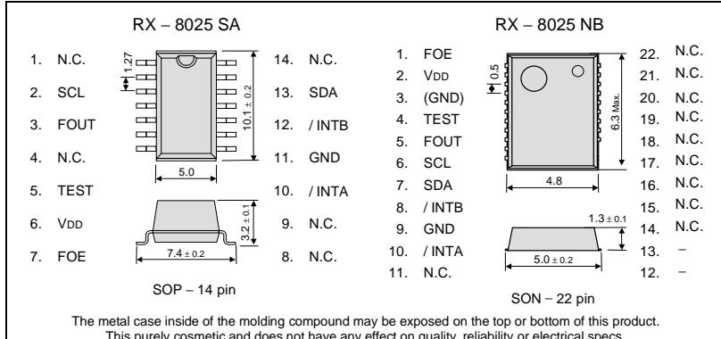
The metal case inside of the molding compound may be exposed on the top or bottom of this product.
