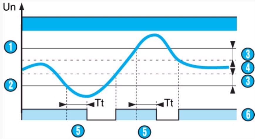
MUSF relays operate in window mode : they check that the controlled voltage stays between a minimum and maximum threshold.
