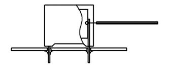
Temperature monitored inside the capacitor.
