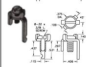
Terminal: .064 Brass-Tin Plated. Screw: Brass - Tin Plated.
