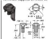
Terminal: .032 Steel, Tin Plated. Screw: Brass - Nickel Plated.
