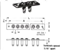
PBE: Paper base electrical, FED. LP-513 Type XP natural, Temp. 250°F max. (121°C) Terminals supplied on these strips
