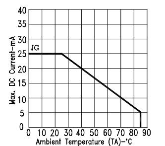
Fig5. MAX. ALLOWABLE DC CURRENT
