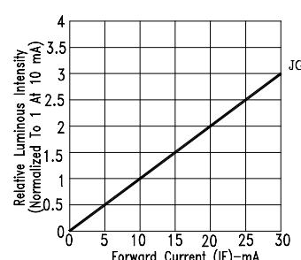
Fig4. RELATIVE LUMINOUS INTENSITY
