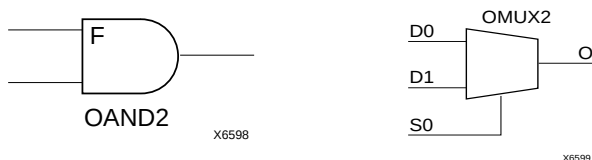
Figure 20: AND & MUX Symbols in XC4000X IOB
