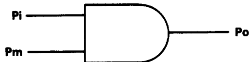
Figure 5. Equivalent Logical Representation of Masking Operation
