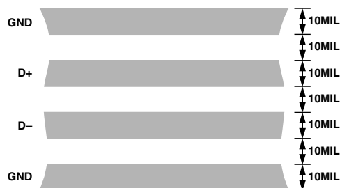
Figure 4. Arrangement of Signal Tracks
