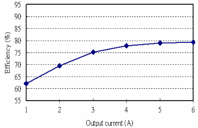
Figure 2: Converter efficiency vs. output current (0.9V output voltage, 12V input voltage)
