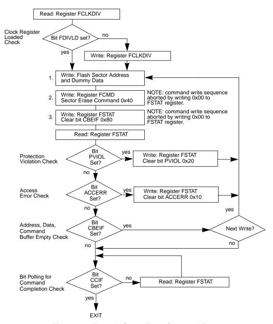
Figure 2-27. Example Sector Erase Command Flow
