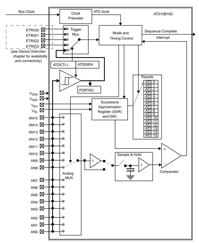
Figure 6-1. ATD10B16C Block Diagram
