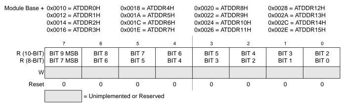
Figure 6-18. Left Justified, ATD Conversion Result Register x, High Byte (ATDDRxH)
