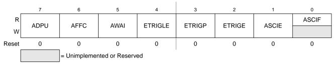
Figure 6-5. ATD Control Register 2 (ATDCTL2)
