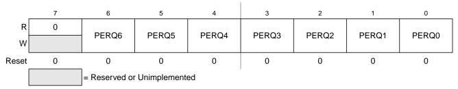
Figure 3-27. Port Q Pull Device Enable Register (PERQ)
