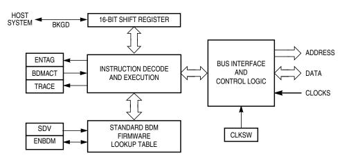
Figure 15-1. BDM Block Diagram
