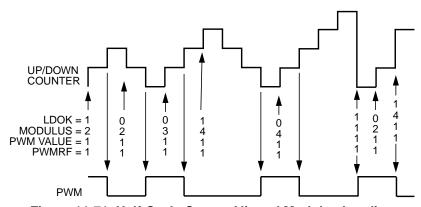
Figure 11-71. Half-Cycle Center-Aligned Modulus Loading
