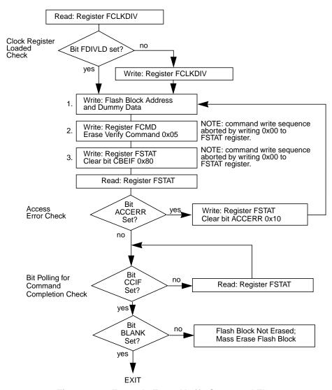
Figure 2-23. Example Erase Verify Command Flow
