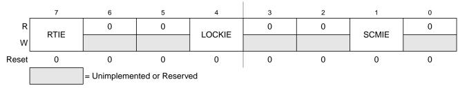
Figure 4-8. CRG Interrupt Enable Register (CRGINT)
