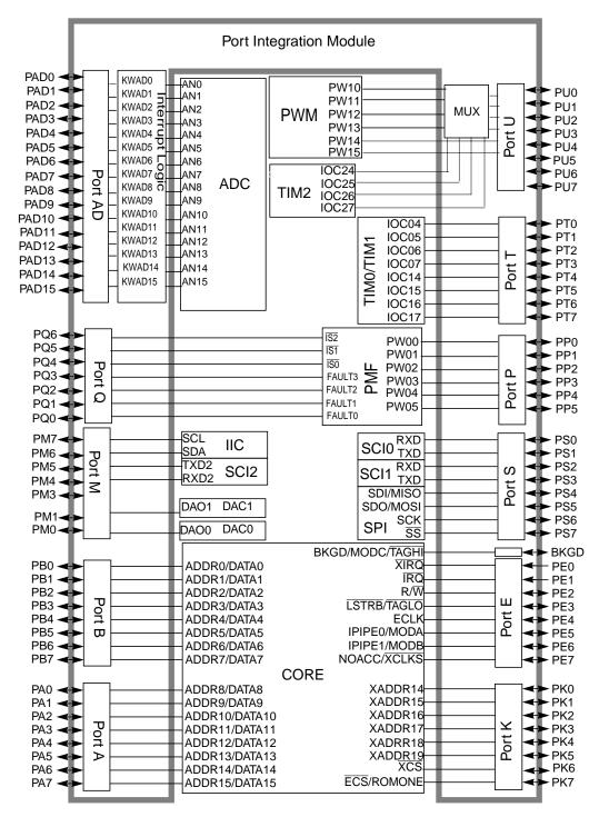
Figure 3-1. PIM9E256V1 Block Diagram
