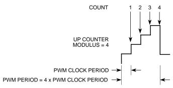
Figure 11-44. Edge-Aligned PWM Period
