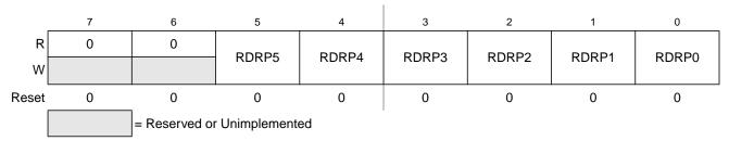
Figure 3-20. Port P Reduced Drive Register (RDRP)
