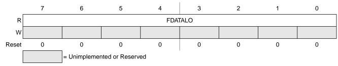
Figure 2-17. Flash Data Low Register (FDATALO)
