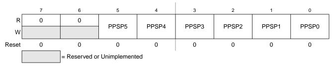
Figure 3-22. Port P Polarity Select Register (PPSP)
