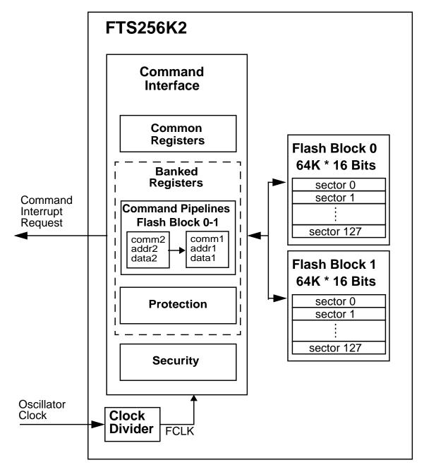
Figure 2-1. FTS256K2 Block Diagram
