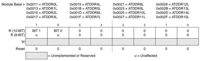
Figure 6-19. Left Justified, ATD Conversion Result Register x, Low Byte (ATDDRxL)
