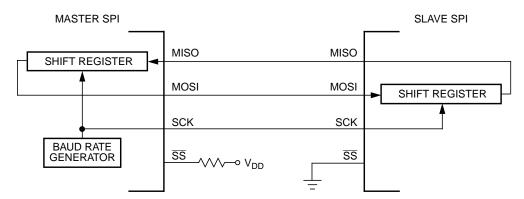
Figure 9-8. Master/Slave Transfer Block Diagram
