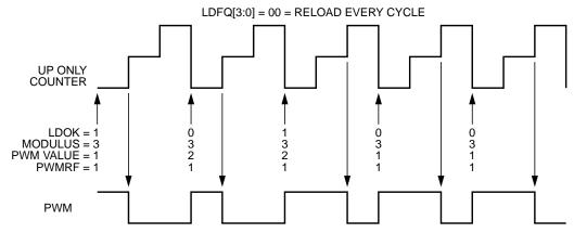
Figure 11-72. Edge-Aligned PWM Value Loading
