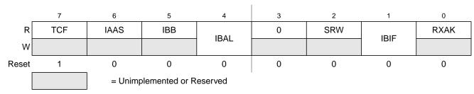
Figure 10-7. IIC Bus Status Register (IBSR)
