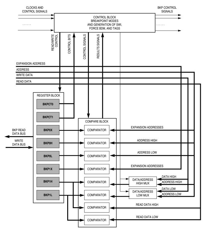
Figure 16-1. DBG Block Diagram in BKP Mode
