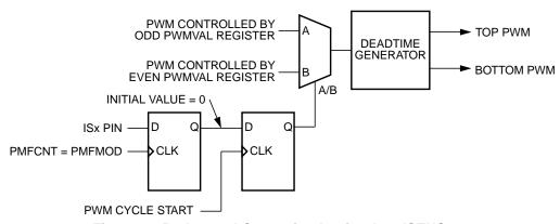
Figure 11-58. Internal Correction Logic when ISENS = 11
