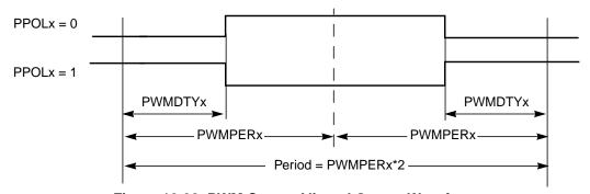
Figure 12-38. PWM Center Aligned Output Waveform
