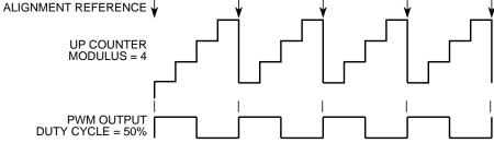
Figure 11-42. Edge-Aligned PWM Output
