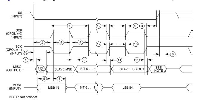
Figure A-7. SPI Slave Timing (CPHA = 0)
