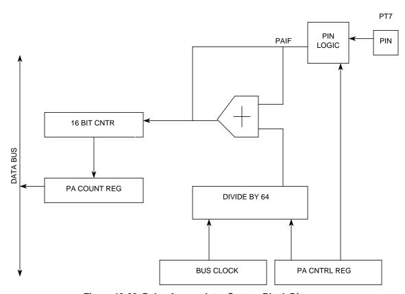
Figure 13-22. Pulse Accumulator System Block Diagram
