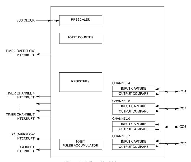
Figure 13-1. Timer Block Diagram
