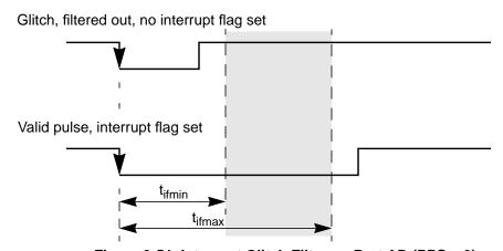
Figure 3-51. Interrupt Glitch Filter on Port AD (PPS = 0)
