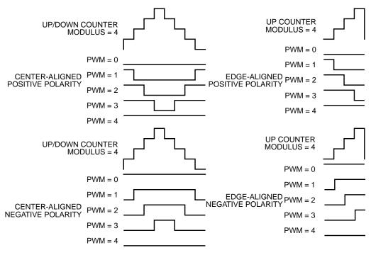
Figure 11-61. PWM Polarity
