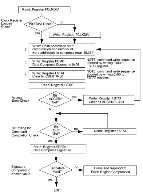
Figure 2-24. Example Data Compress Command Flow
