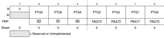
Figure 3-23. Port Q I/O Register (PTQ)
