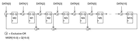
Figure 2-25. 16-Bit MISR Diagram
