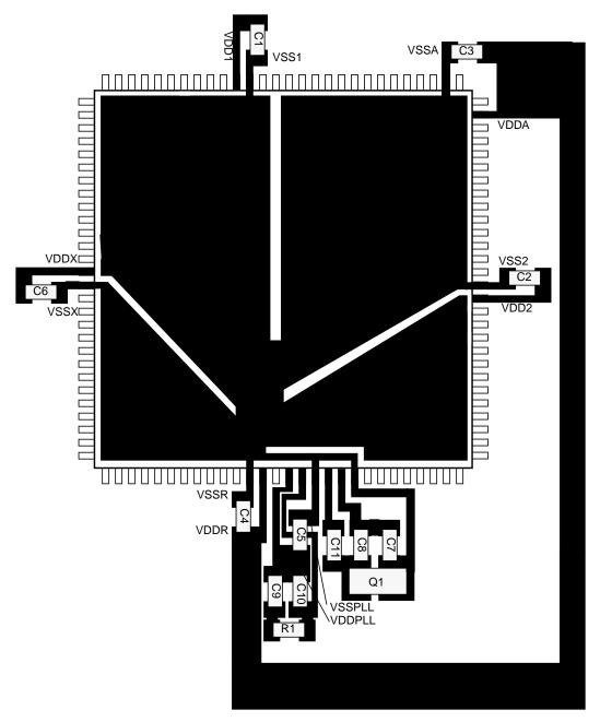
Figure 1-8. Recommended PCB Layout (112-LQFP)
