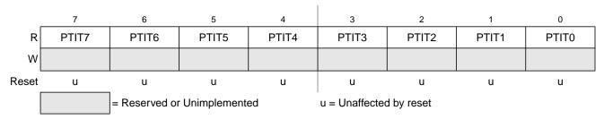
Figure 3-37. Port T Input Register (PTIT)
