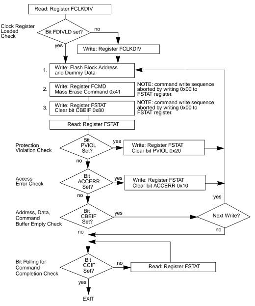
Figure 2-28. Example Mass Erase Command Flow
