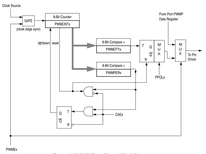
Figure 12-35. PWM Timer Channel Block Diagram
