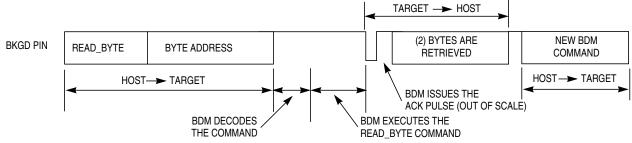
Figure 15-11. Handshake Protocol at Command Level
