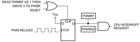
Figure 11-67. PWMRF Reload Interrupt Request
