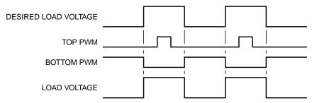
Figure 11-60. Correction with Negative Current
