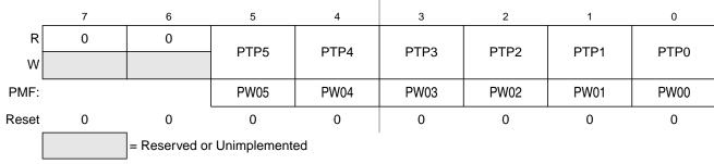
Figure 3-17. Port P I/O Register (PTP)
