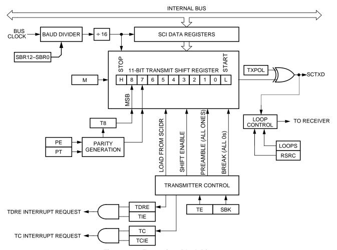
Figure 8-13. Transmitter Block Diagram
