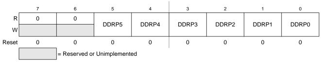
Figure 3-19. Port P Data Direction Register (DDRP)
