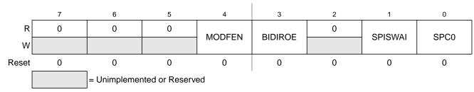
Figure 9-4. SPI Control Register 2 (SPICR2)
