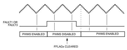
Figure 11-79. Manual Fault Clearing (Faults 1 and 3)
