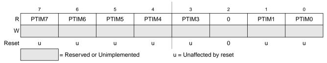
Figure 3-11. Port M Input Register (PTIM)
