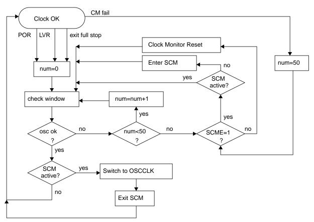
Figure 4-20. Sequence for Clock Quality Check
