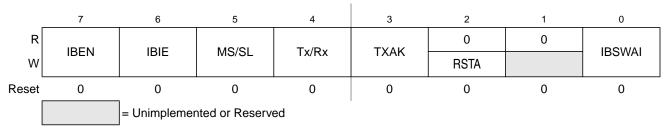
Figure 10-6. IIC Bus Control Register (IBCR)
