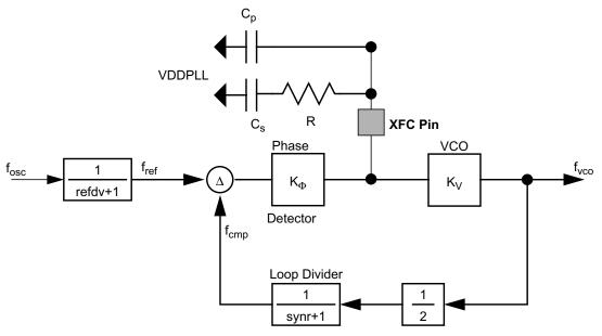
Figure A-2. Basic PLL Functional Diagram
