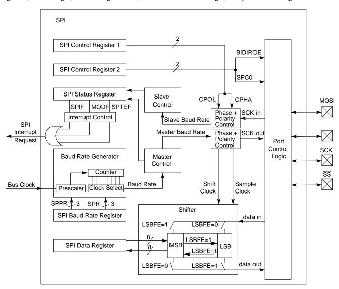
Figure 9-1. SPI Block Diagram
