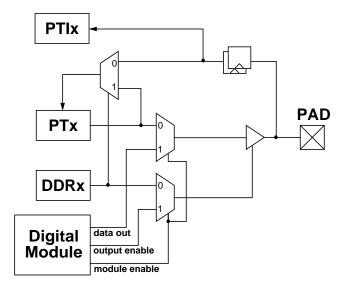
Figure 3-49. Illustration of I/O Pin Functionality
