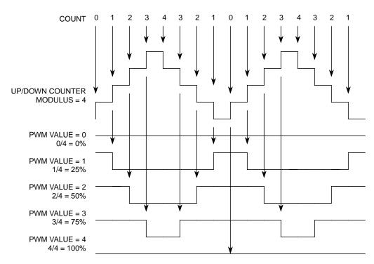
Figure 11-45. Center-Aligned PWM Pulse Width
