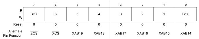
Figure 18-19. Port K Data Register (PORTK)
