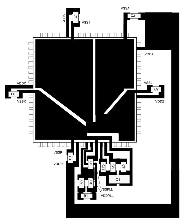
Figure 1-9. Recommended PCB Layout (80-QFP)
