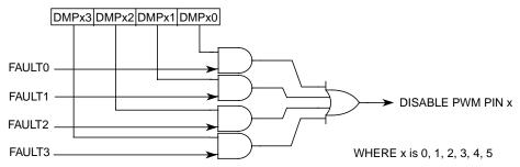
Figure 11-15. Fault Decoder
