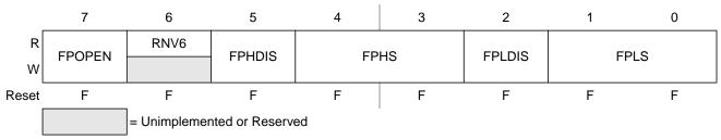
Figure 2-8. Flash Protection Register (FPROT)
