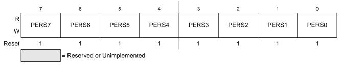
Figure 3-33. Port S Pull Device Enable Register (PERS)
