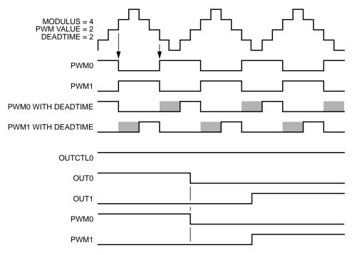
Figure 11-63. Clearing OUT0 with OUTCTL Set In Complementary Mode
