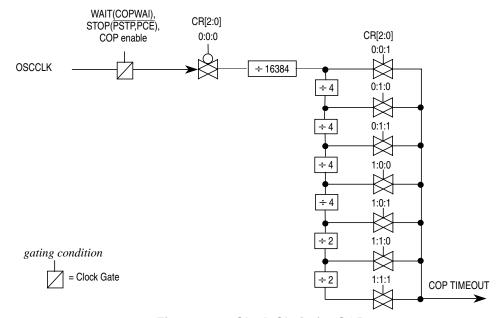
Figure 4-21. Clock Chain for COP
