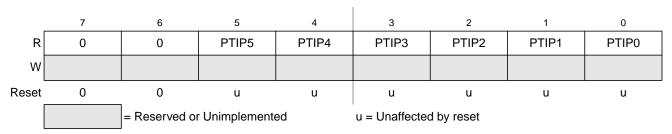
Figure 3-18. Port P Input Register (PTIP)
