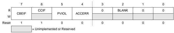
Figure 2-10. Flash Status Register (FSTAT - Normal Mode)
