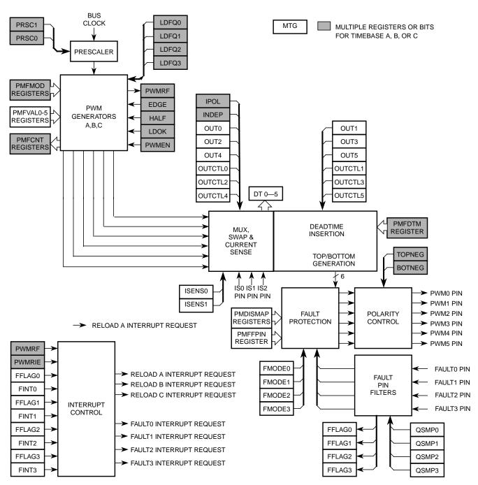
Figure 11-1. PMF Block Diagram
