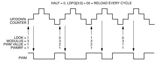
Figure 11-68. Full-Cycle Center-Aligned PWM Value Loading
