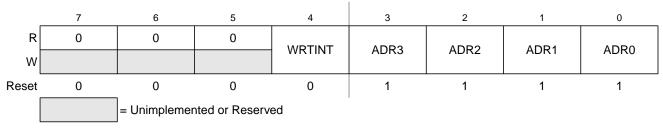
Figure 17-2. Interrupt Test Control Register (ITCR)
