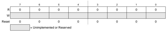
Figure 4-6. CRG Reserved Register (CTFLG)
