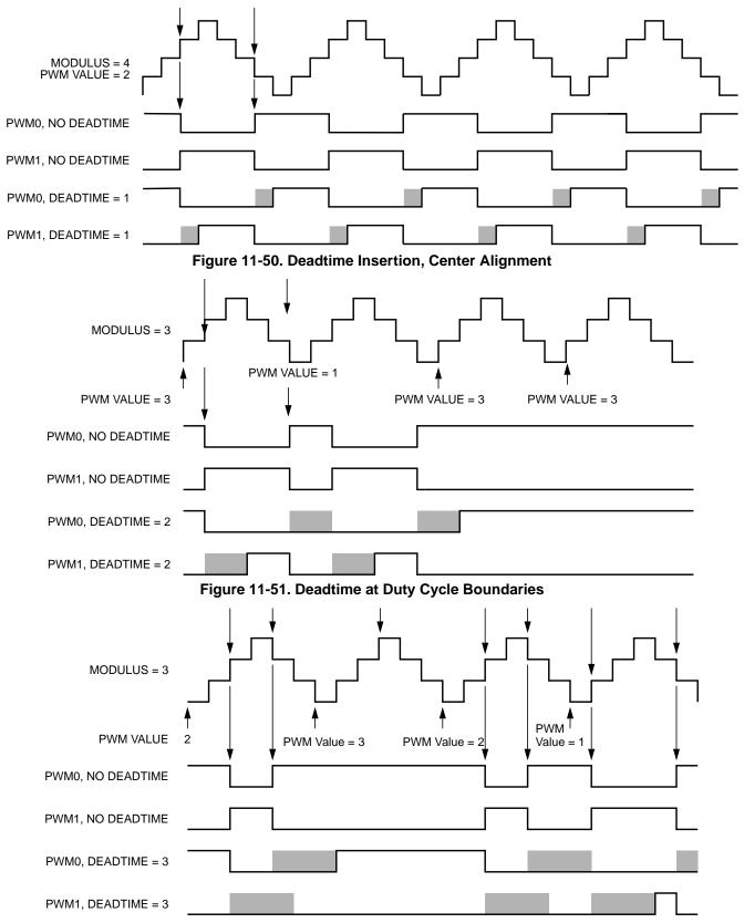
Figure 11-52. Deadtime and Small Pulse Widths
