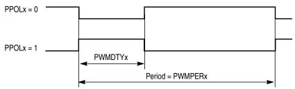
Figure 12-36. PWM Left Aligned Output Waveform
