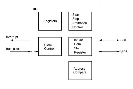
Figure 10-1. IIC Block Diagram
