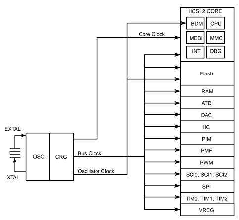
Figure 1-7. Clock Connections
