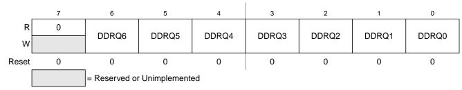
Figure 3-25. Port Q Data Direction Register (DDRQ)
