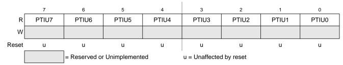
Figure 3-43. Port U Input Register (PTIU)
