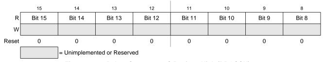
Figure 16-11. Debug Comparator C Register High (DBGCCH)
