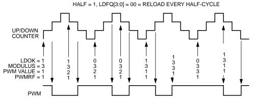
Figure 11-70. Half-Cycle Center-Aligned PWM Value Loading
