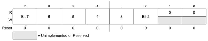
Figure 18-11. Data Direction Register E (DDRE)
