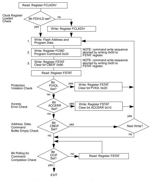
Figure 2-26. Example Program Command Flow
