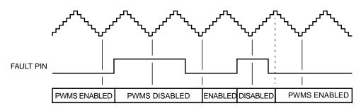
Figure 11-76. Automatic Fault Clearing
