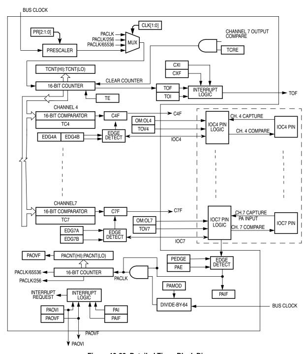
Figure 13-20. Detailed Timer Block Diagram
