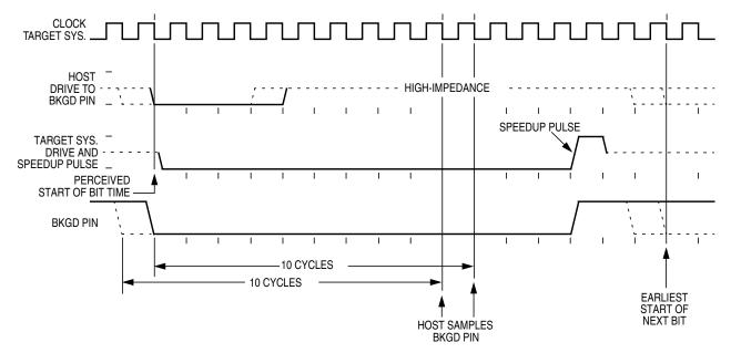
Figure 15-9. BDM Target-to-Host Serial Bit Timing (Logic 0)
