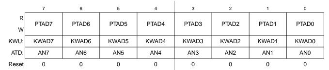
Figure 3-2. Port AD I/O Register (PTAD)
