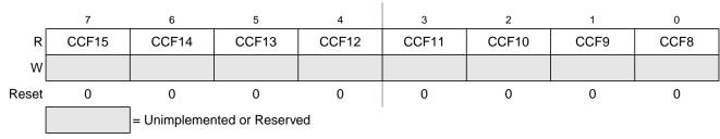
Figure 6-12. ATD Status Register 2 (ATDSTAT2)
