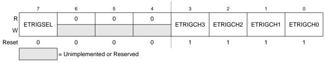
Figure 6-4. ATD Control Register 1 (ATDCTL1)
