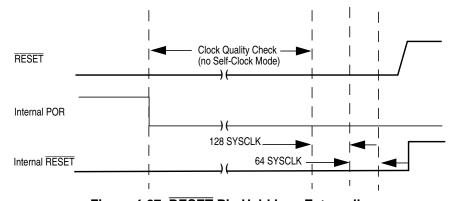
Figure 4-27. RESET Pin Held Low Externally
