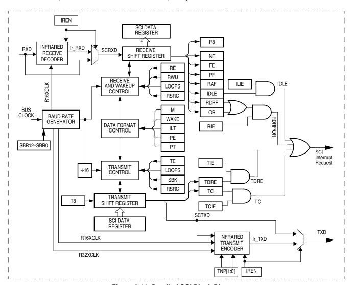
Figure 8-11. Detailed SCI Block Diagram
