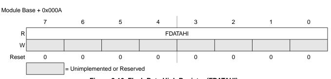
Figure 2-16. Flash Data High Register (FDATAHI)
