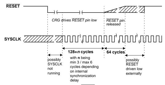
Figure 4-25. RESET Timing
