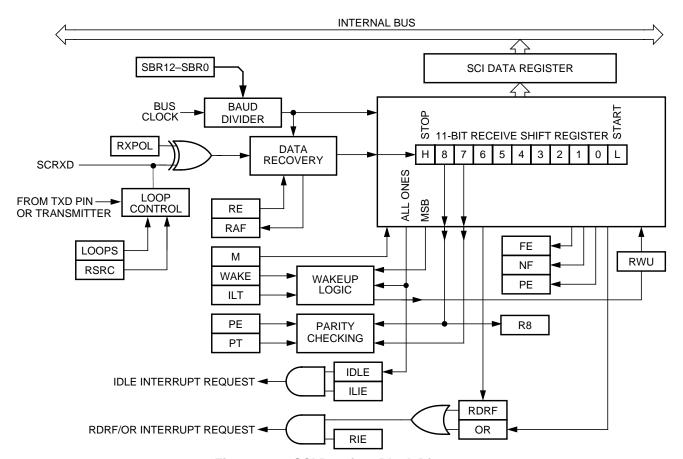
Figure 8-14. SCI Receiver Block Diagram
