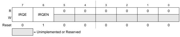
Figure 18-18. IRQ Control Register (IRQCR)
