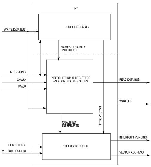
Figure 17-1. INTV1 Block Diagram
