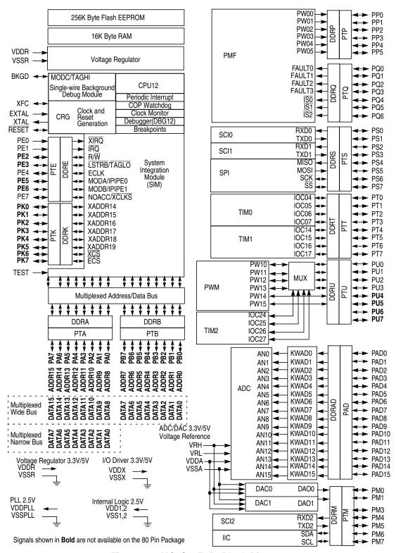
Figure 1-1. MC9S12E256 Block Diagram
