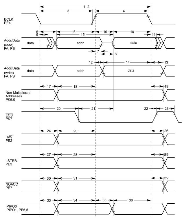
Figure A-10. General External Bus Timing
