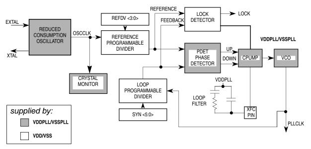
Figure 4-16. PLL Functional Diagram
