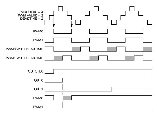
Figure 11-62. Setting OUT0 with OUTCTL Set in Complementary Mode
