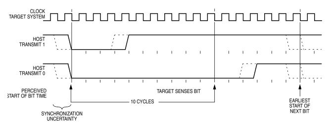
Figure 15-7. BDM Host-to-Target Serial Bit Timing
