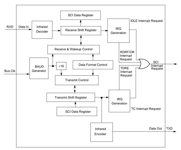
Figure 8-1. SCI Block Diagram
