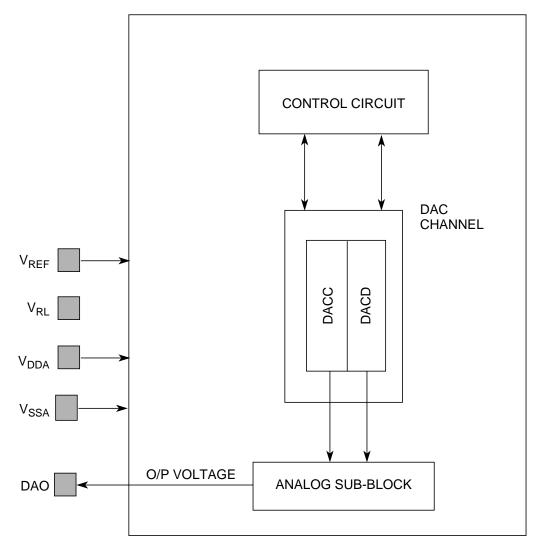
Figure 7-1. DAC8B1C Functional Block Diagram
