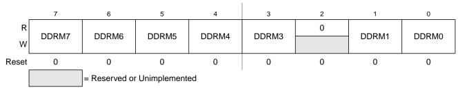
Figure 3-12. Port M Data Direction Register (DDRM)
