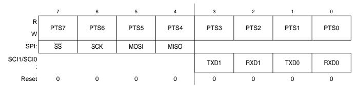
Figure 3-29. Port S I/O Register (PTS)
