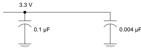
Figure 9-2. Recommended M-LVDS Bypass Capacitor Layout
