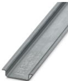
DIN rail, unperforated, Standard profile, width: 35 mm, height: 7.5 mm, In acc. with EN 60715: 2001, material: Steel, galvanized, length: 2000 mm, color: silver
