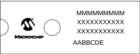
40-Lead CERDIP Windowed
