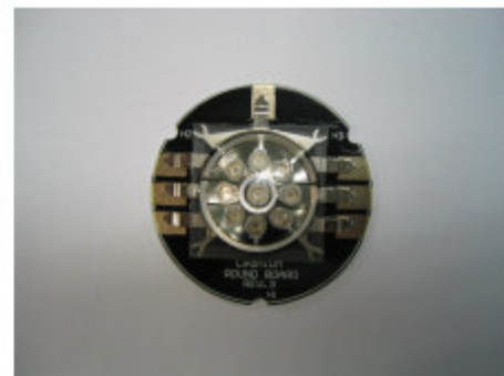
Test set-up on MCPCB
