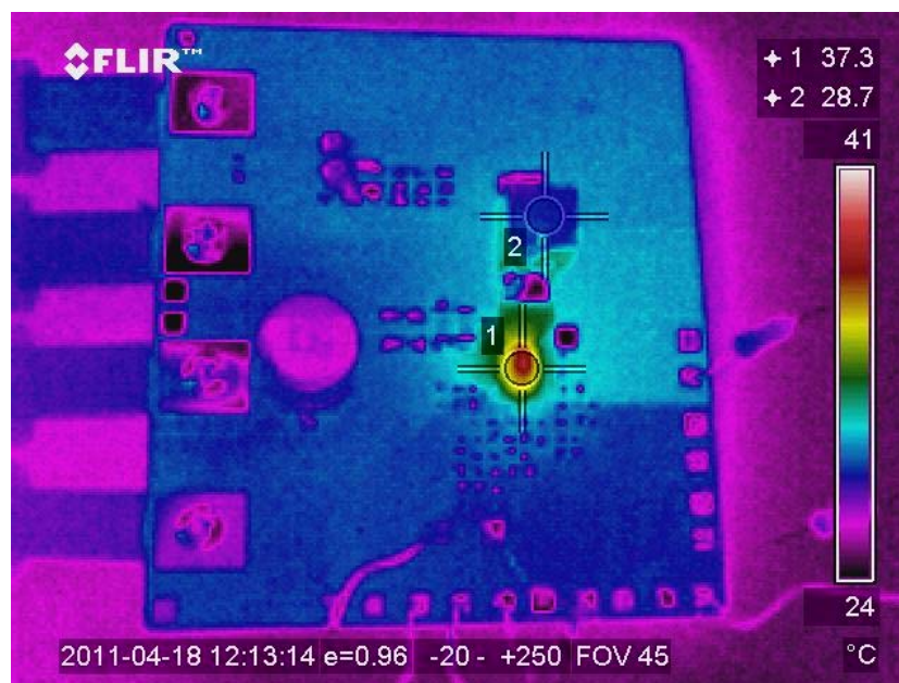
Figure 42: Thermal Image of the Board at 4A Load, Test Point 1 is IR3897, Test Point 2 is inductor
