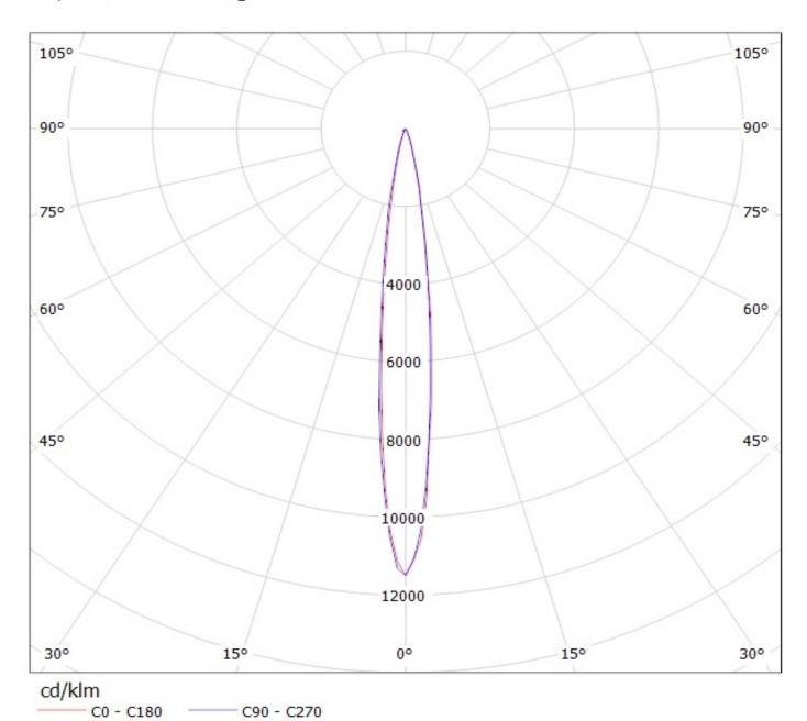
Luminaire: Ledil Oy CA12666\_LXB2-M (Cree XB-D 84lm @ 250mA) LOR=81% Lamps: 1 x Cree XB-D 84lm @ 250mA
