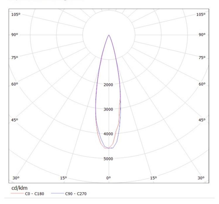
Luminaire: Ledil Oy CA12667\_LXB2-W (Cree XB-D 84Im @ 250mA) LOR=81% Lamps: 1 x Cree XB-D 84Im @ 250mA
