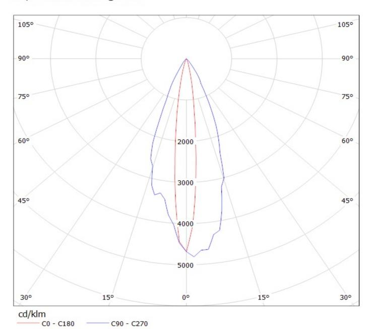
Luminaire: Ledil Oy CA12665\_LXB2-D (Cree XB-D 84lm @ 250mA) LOR=80% Lamps: 1 x Cree XB-D 84lm @ 250mA
