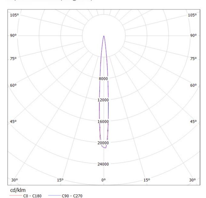
Luminaire: Ledil Oy CA12844\_LXB2-O-90 (Cree XB-D 84Im @ 250mA) LOR=80% Lamps: 1 x Cree XB-D 84Im @ 250mA
