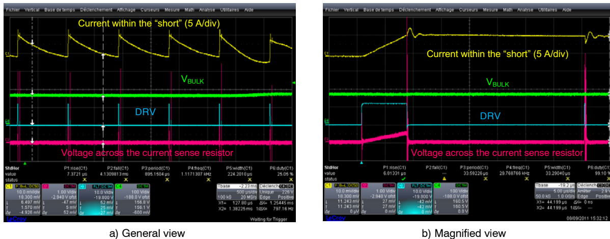
Figure 18. Shorting the Bypass Diode and the NTC
