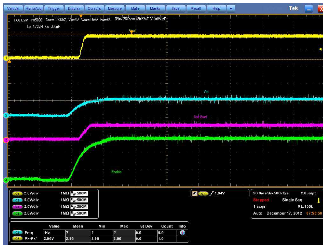
Figure 14. TPS50601SPEVM Start-Up Relative to V_{IN}
