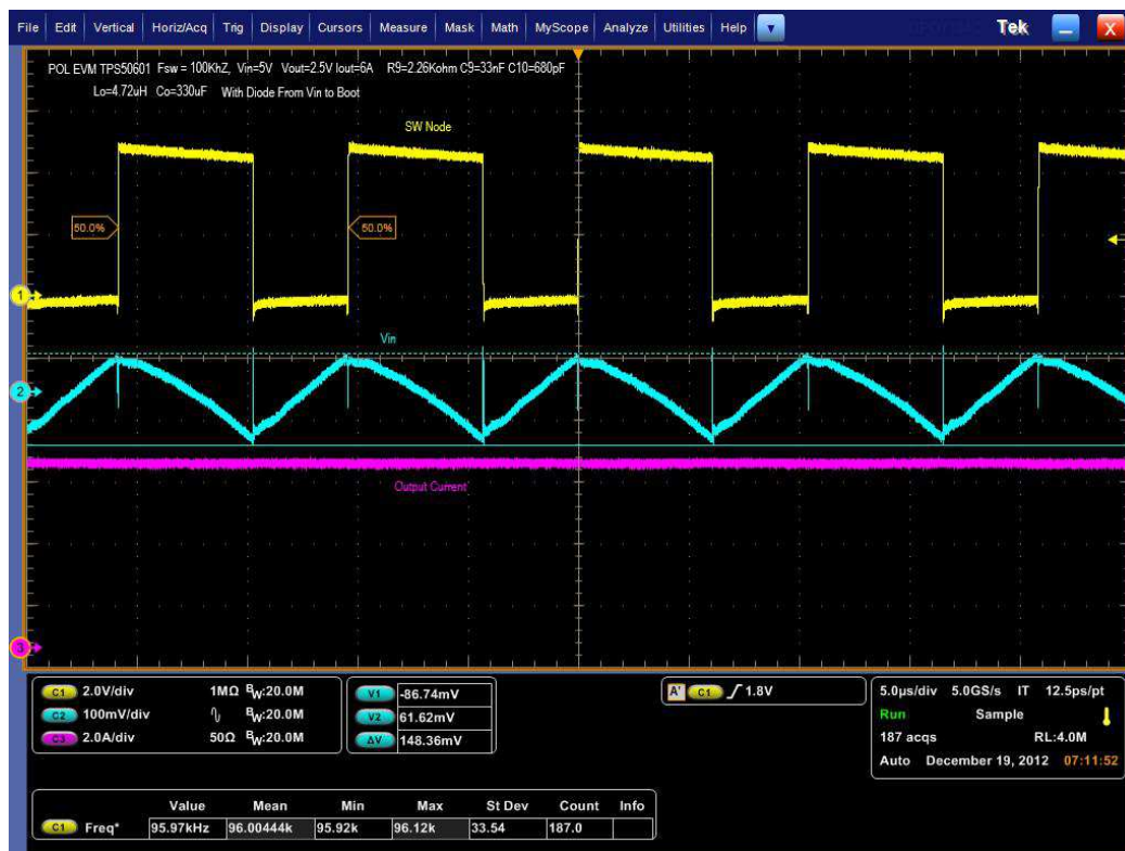
Figure 11. TPS50601SPEVM Input Ripple
