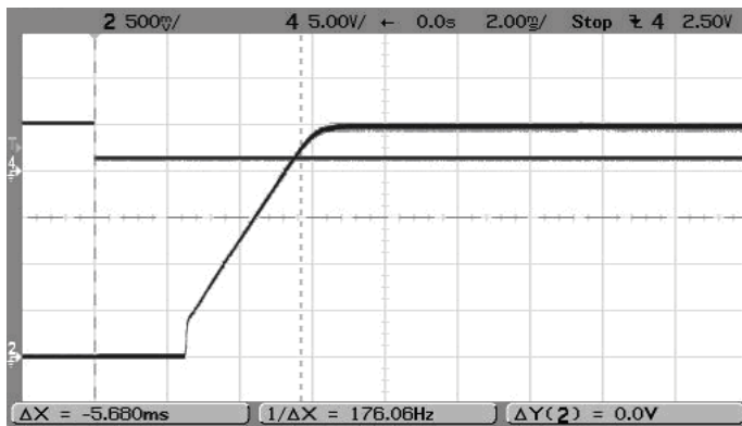
On/Off Enable Delay (Vin=12V, Vout=2.5V, Iout=6A, Load=0) Trace 4=Enable, Trace2=Vout
