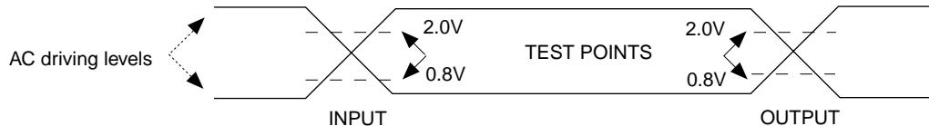
AC TESTING: AC driving levels are 2.4V/0.4V for commercial grade.
